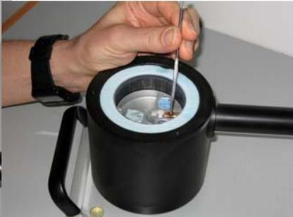
Keep the grid close to the metal surface of the workstation insert during the loading process.
