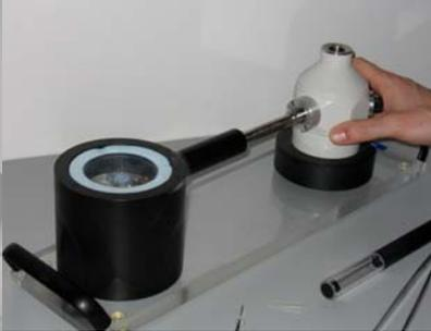
Using pre-cooled large tweezers, quickly transfer the cryo grid box containing the frozen hydrated grids to the liquid nitrogen in the workstation.
