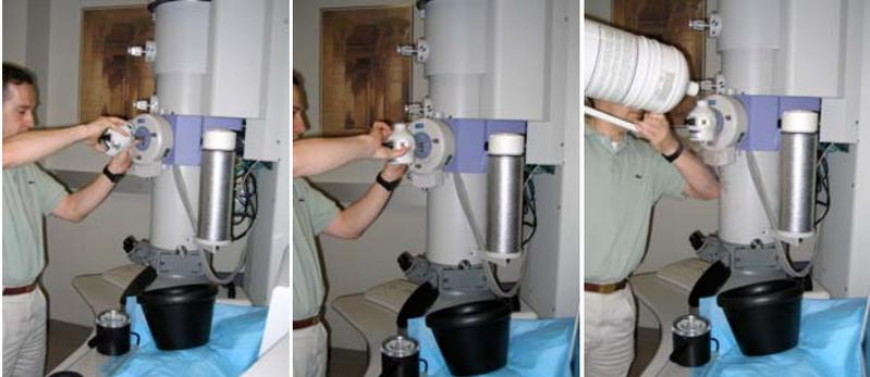
Rotate the holder into position for insertion into the high vacuum of the column and then refill the dewar for the cryo holder. Depending upon the characteristics of the stage mechanism of the microscope that you are using, you may have to wait from 15 – 45 minutes for the holder to thermally equilibrate before recording images.
