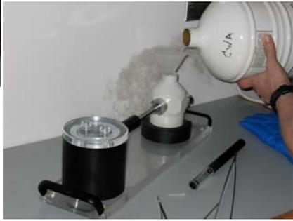
Avoid spilling the liquid nitrogen by using the trapped funnel that comes with the workstation.
