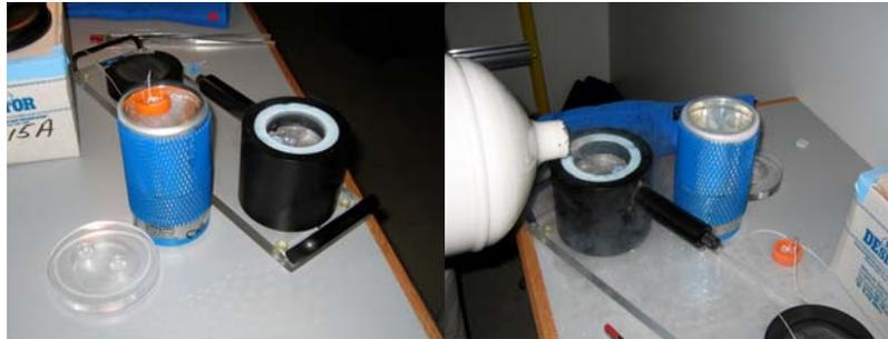
Conical tube with cryo grid boxes in transfer dewar filled with liquid nitrogen.
