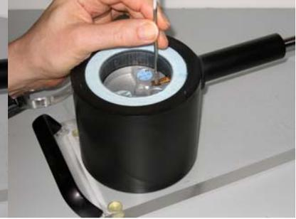
Pre-cool the opposite end of the clip ring tool and then press it gently against the clip ring to ensure that the clip ring is firmly seated in place.
