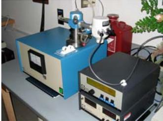
Gatan 626 cryo transfer holder, 655 turbo pumping station and SmartSet 900 Cold Stage Controller
