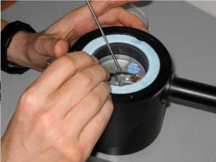
The 70° cryo transfer holder has a special tool to remove the clip ring that holds the specimen grid in place. Insert the tool over the clip ring and rotate the knob at the end of the tool. This action will cause the metal blades located at the opposite end of the tool to engage the clip ring. Once firmly attached, tilt the tool sideways to disengage the clip ring.
