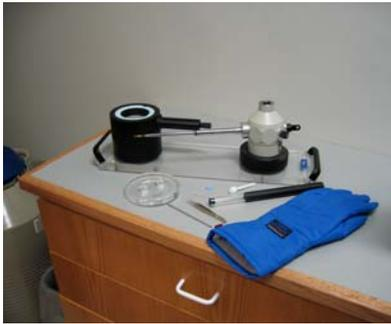
Gatan 626 70° cryo transfer holder, workstation and cover, blue cryo grid box, clip ring tool, fine tweezers, cryo gloves (plug for the workstation is inserted.)
