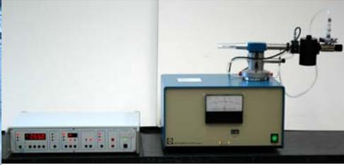
Gatan UK CT3500 cryo transfer holder, ITC temperature controller and 655 turbo pumping station with pump-out adapter
