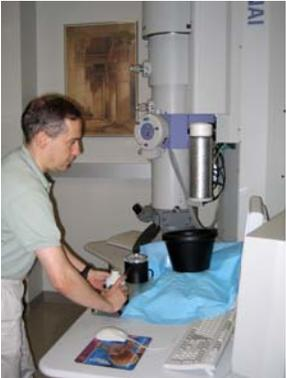
Top of the anti-contaminator. You may want to protect the surface of the microscope.
